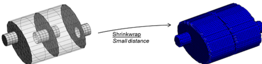
Figure 13.27: Use of the Interior Shrinkwrap function to obtain a closed surface inside a part
